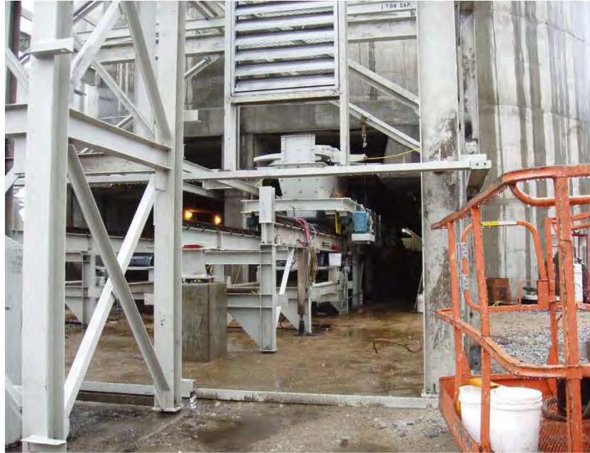
Figure A-9 Limestone rotary plow reclaim equipment set on track inside maintenance area steel
