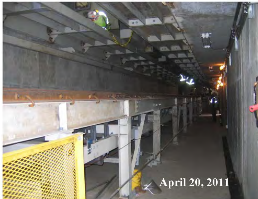
Figure A-9 Steel Reclaim Shelves Above and Rotary Plow Track under Limestone Storage Silos
